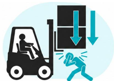
Crushed between forklift and a surface
